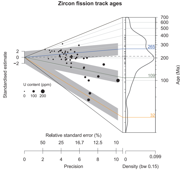
Figure 6: Abanico plot of a set of 50 zircon fission track measurements (sample SH4) published by ?. The plot shows uranium content (in ppm) equal to circle diameter. The data are centered by the weighted mean. The three mean finite mixture components are illustrated by coloured lines.
